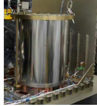
Fig. 7. SHM installed (with holding tool) temporarily into ACES payload
