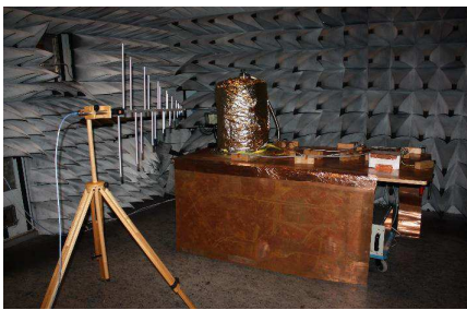
Fig. 6. Test setup inside EMC test chamber for radiated susceptibility test
