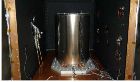
Fig. 4. Test setup in thermal vacuum chamber
